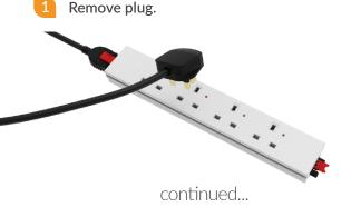
Confirm the red indicator beneath the plug is visible.
