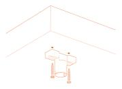
Position the weighted floor mount (noting the position of the cable entry) and connect the required amount of links, ending with the final connection to the desk mount.
